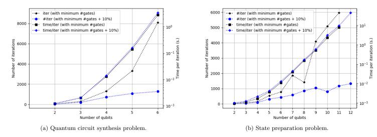
Fig. 4: Number of iterations and time per iteration for different problem sizes.
