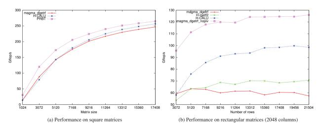
Figure 5: Performance on AMD + Tesla 2050, 16 threads
